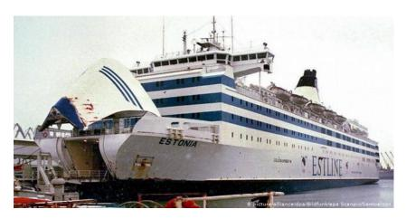
That is with the visor up and the second door open. So that fools you into thinking that if the visor fails in a storm, the ship is toast. But here we see the visor up and the second door closed:
